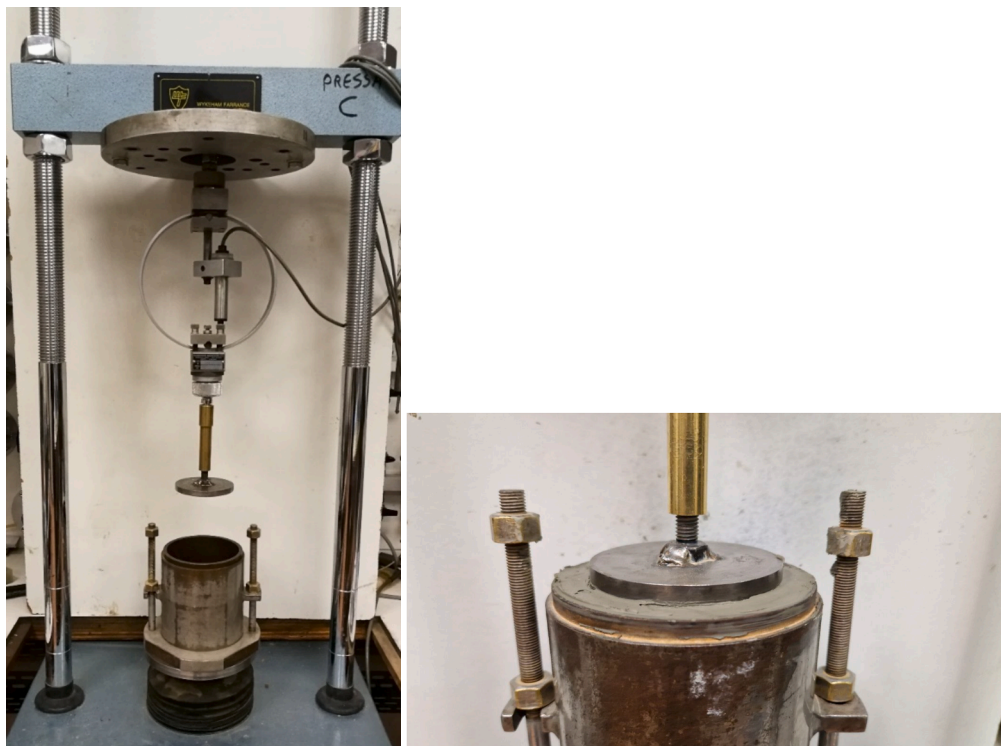
Fig. 4. Pull-out test device with modified convex tool and detail of the plate-soil contact.
