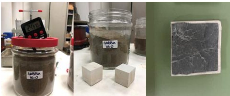
Figure 4. Curing in soil. Aspect of the internal surface of a sample showing external discoloring.
