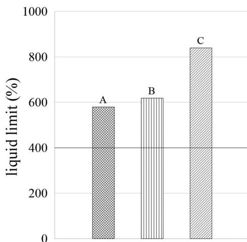
Figure 1. Liquid limit of the bentonite fluids based on natural bentonite (A), extended with natural polymer (B) and extended with synthetic polymer (C).
