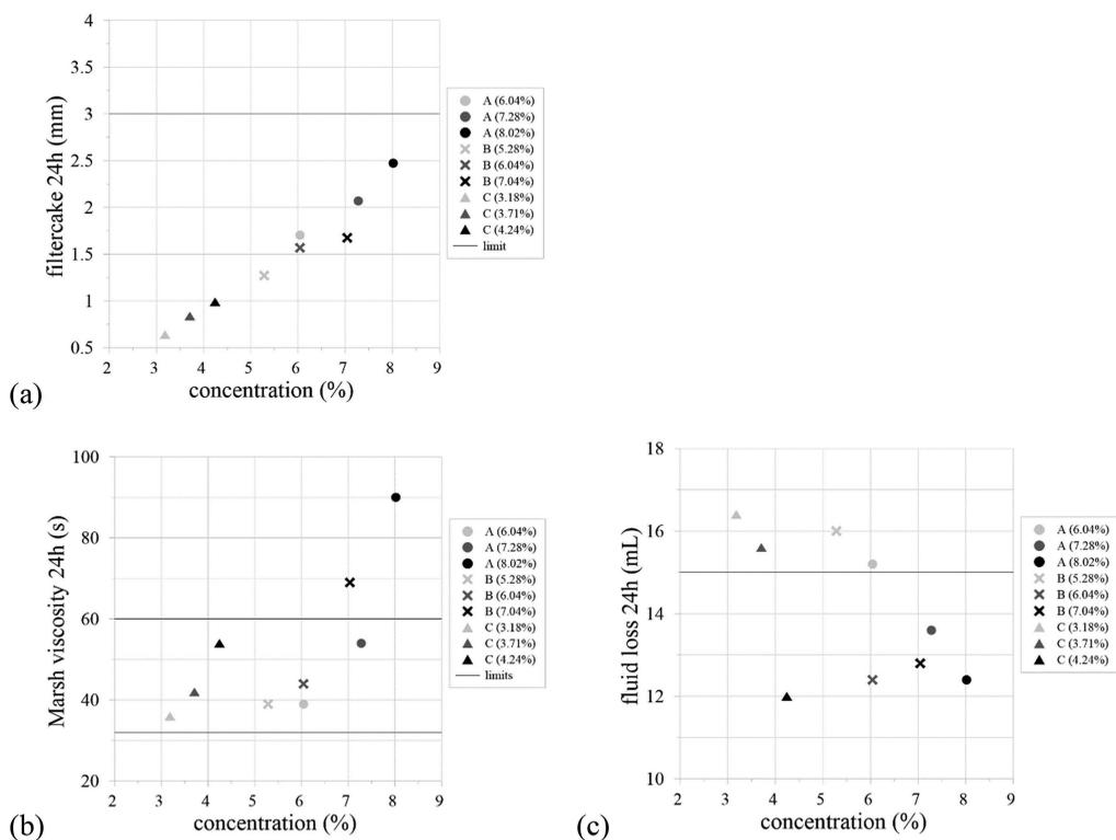
Figure 2. (a) Marsh viscosity, (b) filtercake and (c) fluid loss of bentonite fluids after 24 h.
